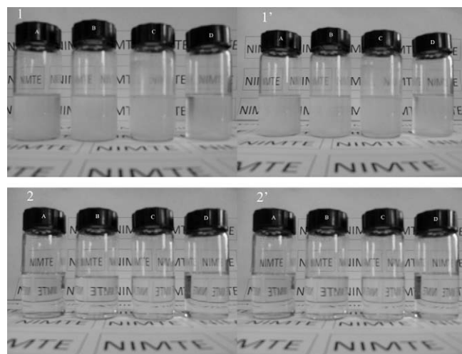
Fig. 1. Pictures of solubility tests: (1) starch nanocrystals and (2) acetylated starch nanocrystals (DS 2.45) were dissolved in (A) N,N -dimethylformamide, (B) acetone, (C) carbon tetrachloride and (D) toluene immediately after stopping stirring, (1') starch nanocrystals and (2') acetylated starch nanocrystals were placed 48 h later.
